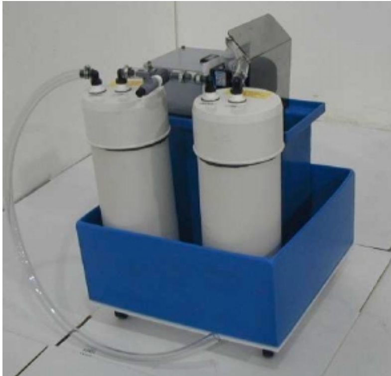
Illustration 1: Hook up Configuration of the Mark 3XE Silver Recovery Unit
