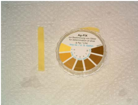
Silver test paper indicates column is performing optimally.
