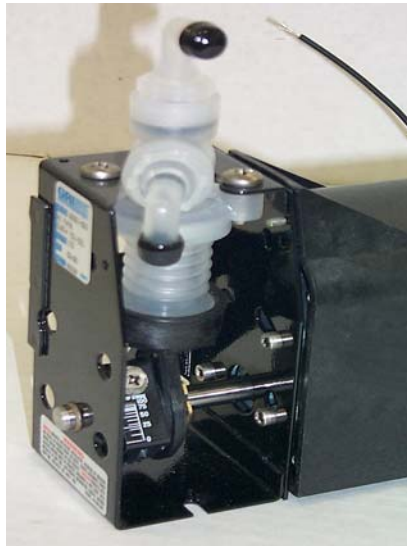
Illustration 4: Calibrating the Pump on the Mark 3X SRU
