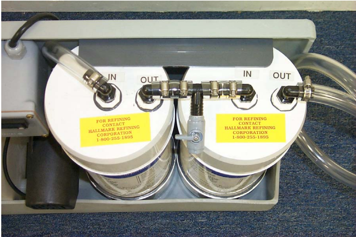
Illustration 1: Hook up Configuration of the Mark 3X Silver Recovery Unit
