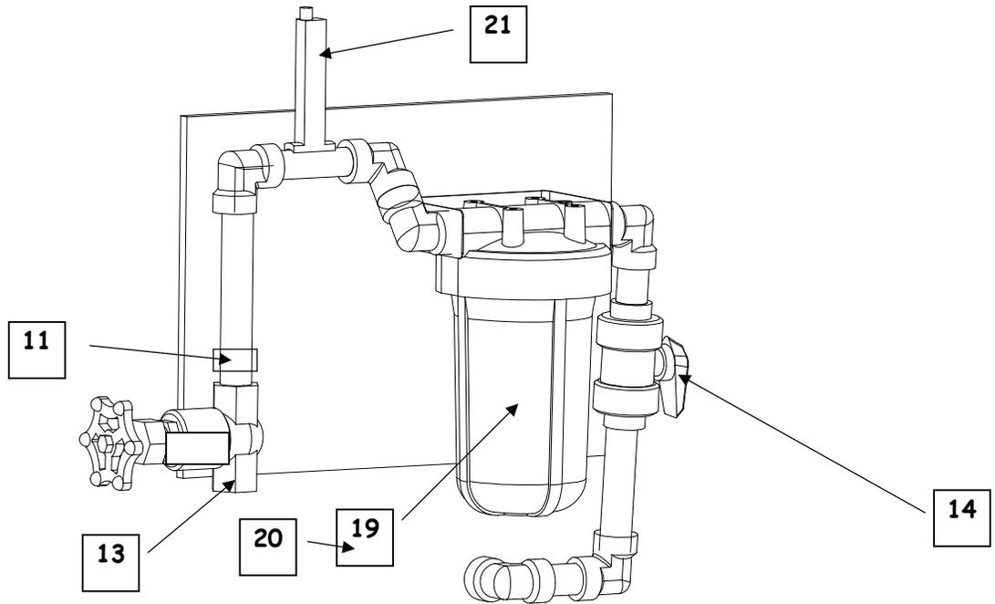
FIGURE 9-3: Flowmeter with Filter Chamber
