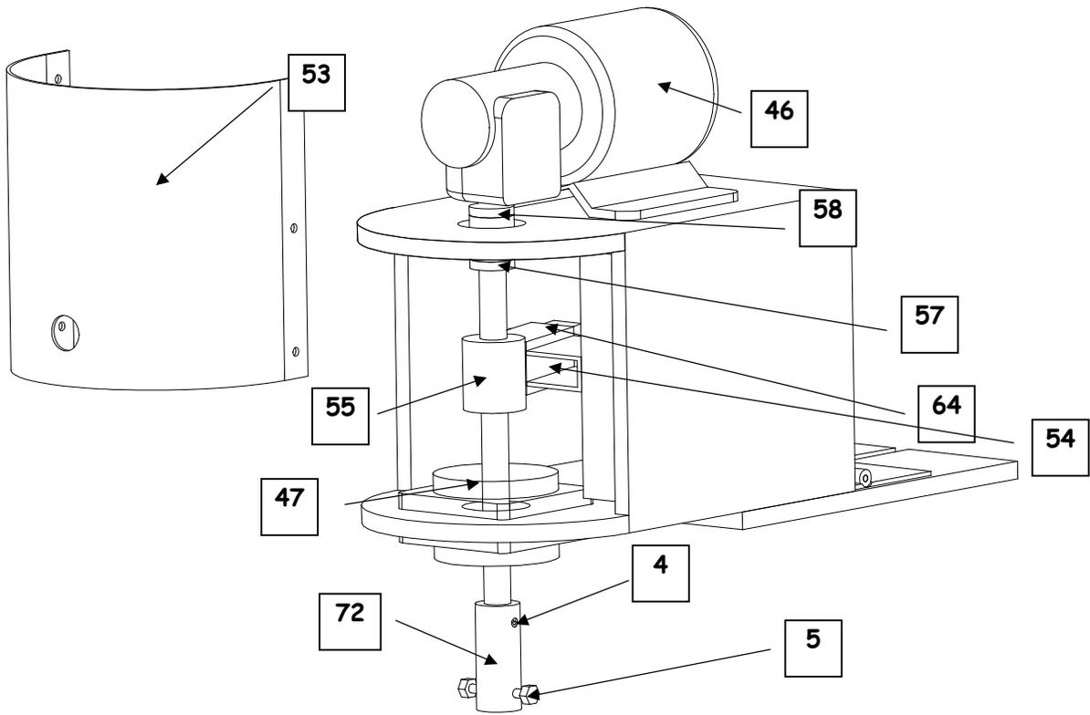
FIGURE 9-8: Drive Assembly Detail #1
