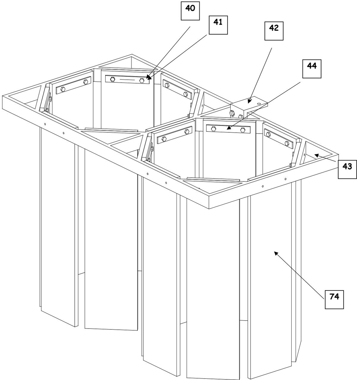
FIGURE 9-5: Anode Ring Assembly
